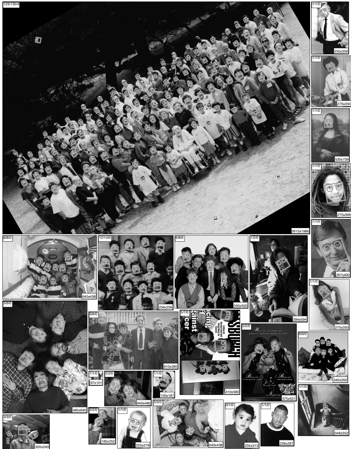
Figure 4.9: Result of arbitrating between two networks trained with derotated negative examples. The label in the upper left corner of each image (D/T/F) gives the number of faces detected (D), the total number of faces in the image (T), and the number of false detections (F). The label in the lower right corner of each image gives its size in pixels.
