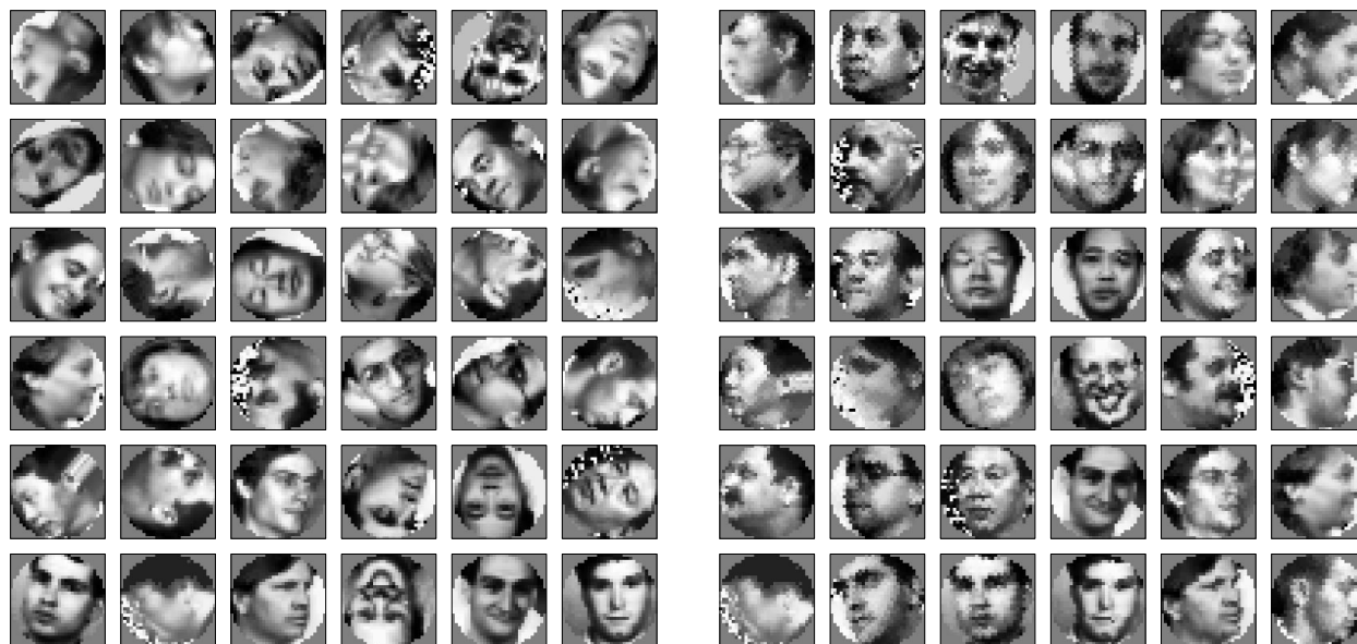
Figure 5.10: Training examples for the category-specific detection networks, as produced by the categorization network. The images on the left are images of random in-plane angles and out-of-plane orientations. The six columns on the right are the results of categorizing each of these images into one of the six categories, and rotating them to an upright orientation. Note that only three category-specific networks will be trained, because the left and right categories are symmetric with one another.
