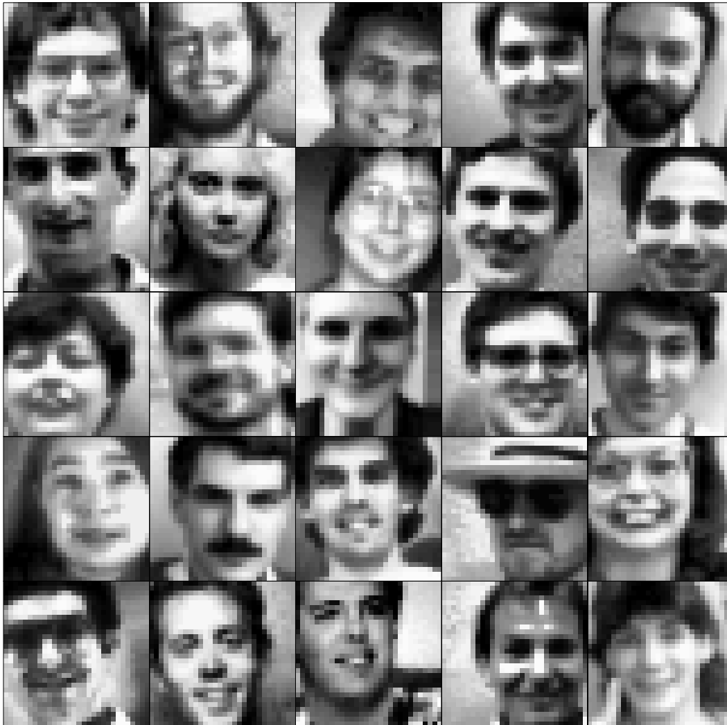
Figure 6.1: Example images used to train the candidate face detector. Each example window is 30 \times 30 pixels, and the faces are as much as five pixels from being centered horizontally and vertically.
