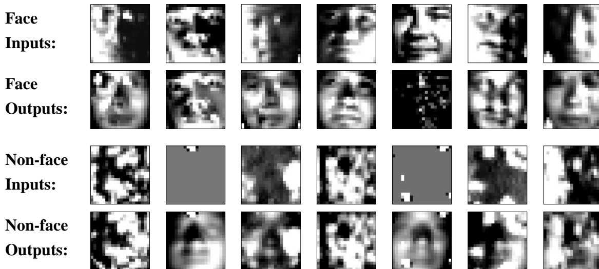
Figure 2.19: Result of lighting correction system. The lighting correction results for most of the faces are quite good, but some of the nonfaces have been changed into faces.
