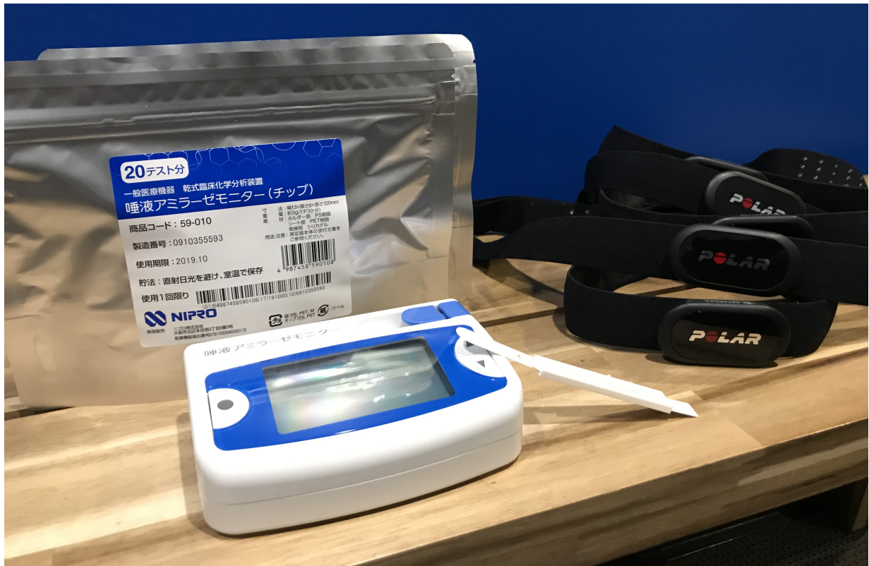
Figure 5.1: Data collection equipment. Left: pouches of saliva swabs. Center: point-of-care salivary amylase meter, with a single saliva swab. Right: Polar H10 cheststrap heart rate monitors.
