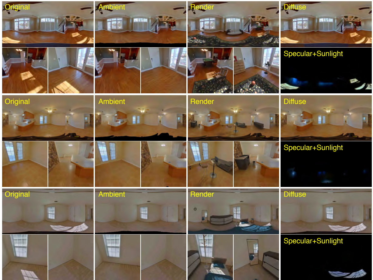
Figure 4.24: Appearance decomposition and object insertion results. The effects (specular + sunlight) are 1.5\times brightened. The perspective samples are shown under the panoramic views of original, ambient, and rendered images. The three examples cover different flooring (wood, tile, carpet) and different effects (both specular and sunlight, specular only, sunlight only). The inserted objects create realistic appearances when blocking specular reflection and the direct sunlight. The direct sunlight is cast upon the inserted objects and further reflected by other surfaces ( e.g. mirror in the bottom example).
