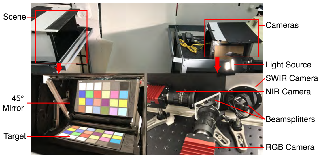
Figure 2.3: Image Acquisition System. RGB, NIR, and SWIR cameras are co-located using beamsplitters. The target is imaged through a 45^\circ mirror.
