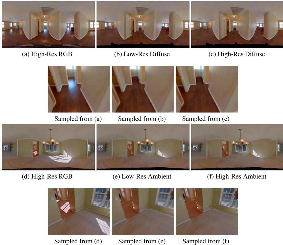
Figure 4.14: Resolution enhancement results. (a)(b)(c) show an example of enhancing specular removal result. The high-res diffuse image (c) increases the resolution of (b), with details consistent with the original image (a). Similarly, (d)(e)(f) show an example where the resolution of sunlight removal result is faithfully enhanced. Note that we focus on the floor region so the sunlight on the walls is outside the scope of the current implementation and thus is not removed.
