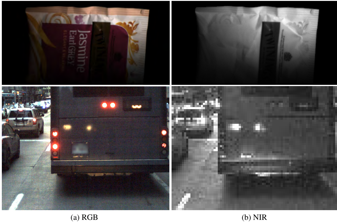
Figure 6.5: Failure cases of “NIR represents shading” assumption. The top row [38] shows that the black pigment strongly absorbs NIR light. The bottom example shows that some LED lights do not emit NIR. In these two cases, NIR intensity is not consistent with RGB shading.
