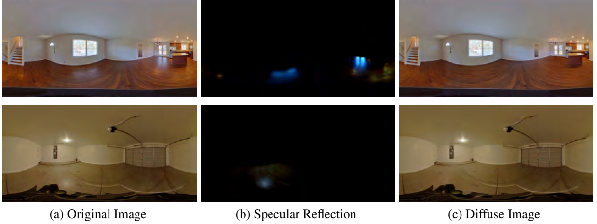
Figure 4.9: Diffuse-specular separation results. Specular reflections are 2\times brightened. Our method handles both strong and weak reflections, from windows and lamps.
