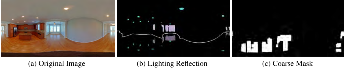
Figure 4.6: Coarse specular reflection mask generation. As in (b), the specular reflection area on a mirror floor is obtained by reflecting the light source (window and lamp) segments. The coarse specular area (c) is generated by further jittering the lamp height and dilating the mask.
