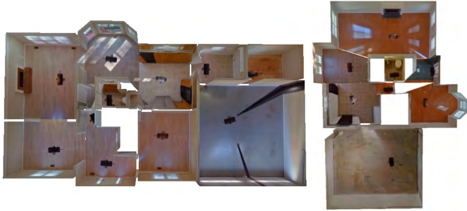
Figure 4.4: 3D visualization of floor layouts. The textures come from projecting panoramas to perspective views. Black artifacts around the centre of each room are tripods.
