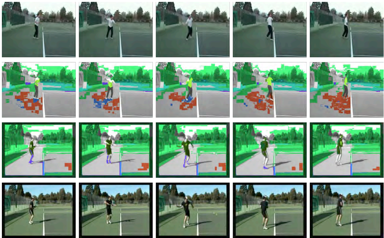
Figure 3.17: Two tennis videos and their matching Motion Words. The two videos are taken in the same environment, but at different locations (courts). The supervoxels corresponding to the players encode to the same Motion Word because they have similar texture and horizontal motion. The supervoxels corresponding to the trees also encode to one Motion Word. Note that the supervoxels corresponding to the ground have different horizontal descriptors due to the shadow of the second player.
