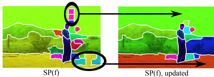
Figure 4.23: For every pair of superpixels that are always neighbors, check if their instantaneous motion is always the same, for all video frames which contain the two superpixels. If this condition is satisfied (e.g. the superpixels pointed to by the arrows), we consider these superpixels as similar in motion, and we merge them in all frames.
