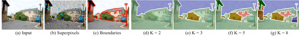
Figure 6.2: An example of segmenting a single image. (a) An input image. (b) 1000 super-pixels and colored evaluation locations \mathcal{L} . (c) Image segmentation with red boundaries. (d)-(g) Color-coded segmentation outputs by ranging K from 2 to 8. As K increases, the following regions are detected in turn: \{\text{sky, tree, wall (center), roof (left), windows (left), building (left), and trash container}\} .
