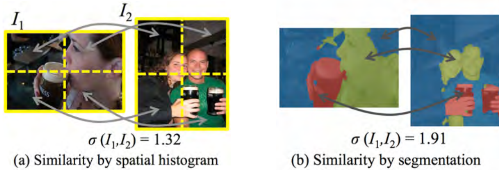
Figure 10.4: The benefit of segmentation for image similarity measurement. (a) For an unsegmented image pair, the spatial pyramid histograms are constructed on the whole images, which may not correctly reflect the location and scale variations. (b) After segmentation, the image similarity is computed as the mean of the best assigned segment similarities.
