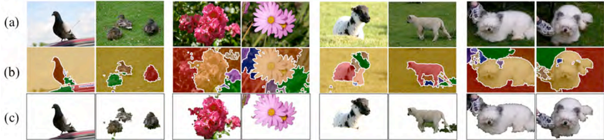
Figure 6.4: Four cosegmentation examples on the MSRC dataset. (a) Pairs of input images. (b) Our cosegmentation results with K=8 . The cosegmented pairs are presented by the same colors. Some segments are too small to be shown. (c) Figure-ground segmentation results that are induced from the eight pairs of cosegments.
