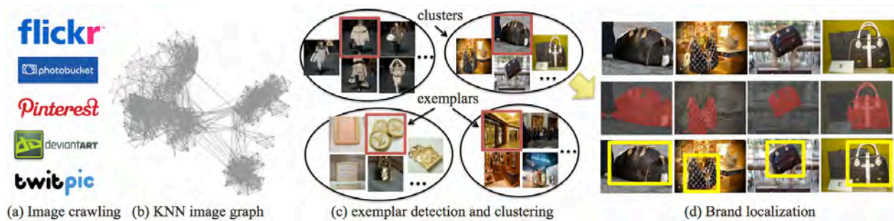
Figure 10.3: The overview of the proposed approach with an example of the Louis+Vuitton . (a) As an input, we crawl the photos of the brand from the five photo sharing sites. (b) Next, we build a K -nearest neighbor (KNN) similarity graph between images. (c) We perform the graph-based exemplar detection/clustering. (d) Finally, we cosegment the images in the same cluster in order to discover the regions of a brand in each image. As a closed-loop solution, we can return to the KNN graph construction with the new segmentation-based image similarity metric.
